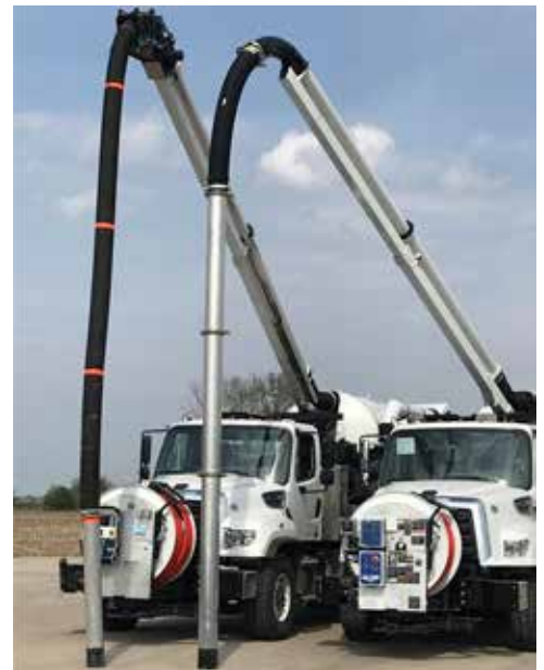
Left unit features the RDB boom and the right unit features the telescopic boom with added tubes.
