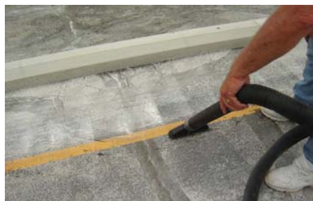
Hand vacuuming remaining simulant on track after sweeping
