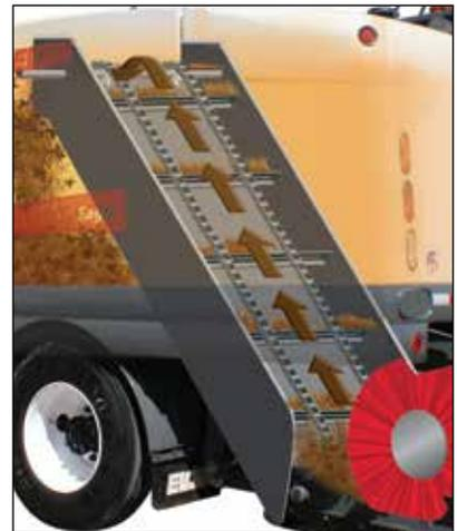
The Eagle conveyors are designed to be interchangeable should a customer have different applications throughout the sweep season.
