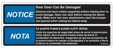
At any time the debris body is raised to obtain access to the underside of the debris body, all safety precautions must be followed. The debris body should be stabilized and secured before entering any space below it. The unit should be parked on a flat level surface.
