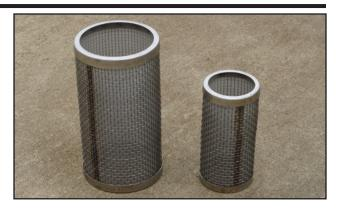
3" Y-strainer on water pump - Disassembled
