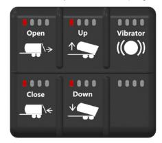
**Return from wireless E-stop:** When in wireless mode and the E-stop on the remote is pressed, trailer latches E-stop until wireless button is pressed again. Wireless indicators flash in sequence.
