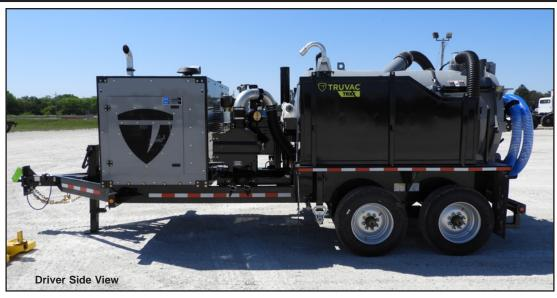
Vacuum Excavation occurs when high-pressure water or pressurized air breaks up and cuts the soil, while a high-flow vacuum system lifts the soil up and out of the excavation area.
