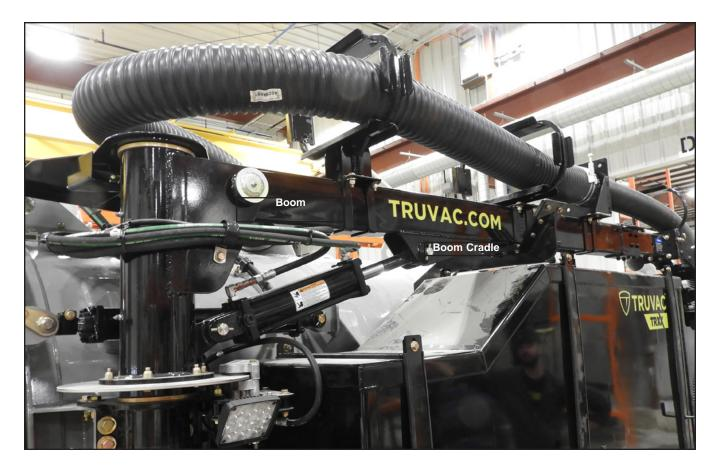
The movement of air by the blower picks up debris and water from the work site and moves the material through a vacuum tube into the debris body. A positive displacement (PD) blower is used to produce the movement of air needed to transport debris from the job site into the debris body. Due to the change in air volume in the debris body, the debris and water are deposited into the body, while air is drawn through ports in the body to the blower where it is exhausted.
