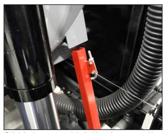
Debris body prop correctly locked in maintenance position.
