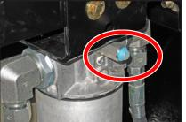
**Note:** besides the typical gauge used on the oil filter housings a second type shown above is used. A red indicator will pop out when ready to be changed.
