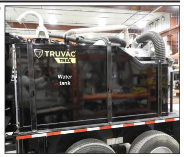
The water tank needs to be filled with clean water before every use. This procedure is the key to extending the life of the pump. Failure to do so may result in pump failure. At the end of each work day, allow the water tank to drain and dry out over night.
