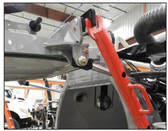
Rear door prop correctly locked in maintenance position.
