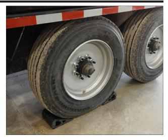
Always chock the wheels to prevent the unit from rolling while working or storing.
