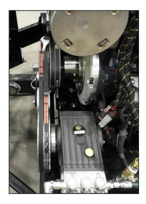
The water system is used to power a high pressure handgun for digging or washing. Capabilities include variable pressure up to a max of 3000 psi at 5gpm. It is only compatible with a special high pressure handgun/high pressure wand. The selected nozzle size, as well as the pressure set with the unloader valve, are what determines the flow rate.
