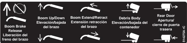
Access to the hydraulic control valve can be had from the passenger side, behind the engine cabinet. This valve allows for manual operation of all hydraulic functions related to the boom and debris body in case of electronic control box malfunction.
