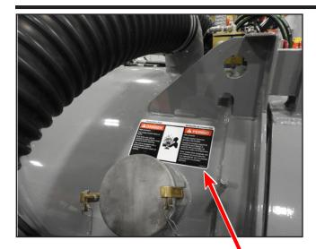
The debris body is equipped with an inspection port on the driver side and is sealed with a cam-lok fitting. It is important to know that the body could be pressurized and the proper procedure must be followed before opening:
