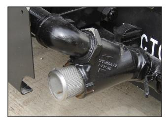
2" Y-strainer at water fill - Disassembled
