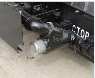
Typical composite Y Strainer. Cap unscrews to remove filter.
