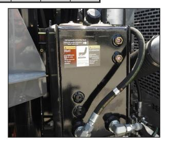
The oil filters supplied by Vactor/Guzzler are equipped with a high efficiency absolute filtering media. Many common filters only give approximately thirty percent filtration of the particles in the hydraulic oil. These filters are referred to as nominal filters. Absolute filtering can give as much as ninety eight percent filtration of the particles in the hydraulic oil. Vactor/Guzzler uses and recommends only the use of absolute filters.
