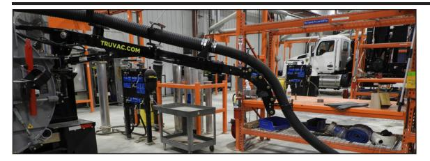
Replacement of the boom hose is made by rotating the boom out towards the rear of the unit so that the boom is aligned/straight with the debris body inlet. Drop the boom down so the hose goes across the boom pivot. This is the longest distance the hose has to make. After removing the old hose verify the new hose is the same as the old one before installing. Failure to utilize the same hose may result in kinking at the bend radius.
