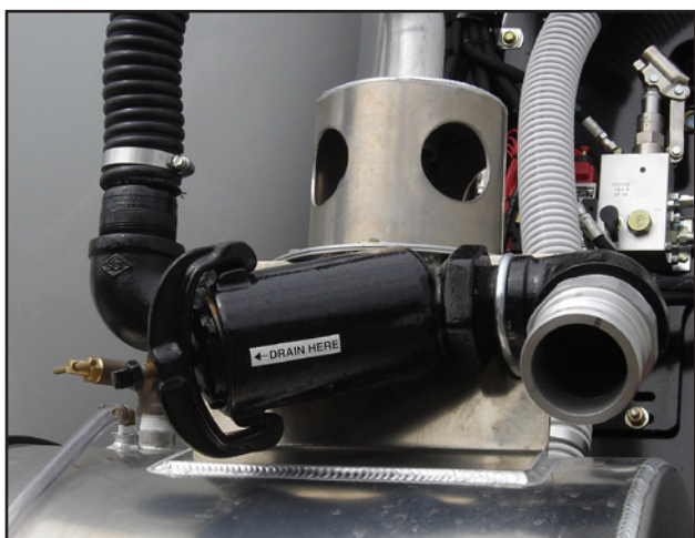
2" Y-strainer at water fill - Assembled
