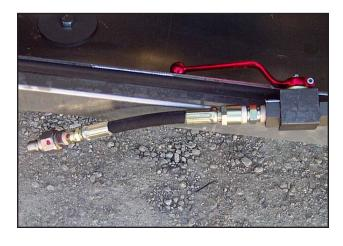
This unit is equipped with a high pressure handgun. The high pressure handgun can only be connected to the hose reel located in the water pump cabinet. The high pressure water system uses up to the full water pump pressure of 3000 psi and can only be used with the special high pressure handgun or a high pressure wand.
