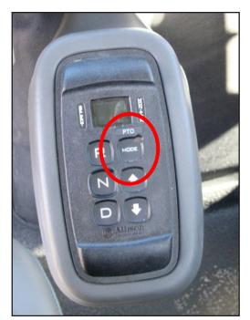
FLXX-C - The MODE switch is normally used on automatic transmissions.
