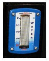
Water level - A gauge is located on sides of the unit normally in front of the watertanks.
