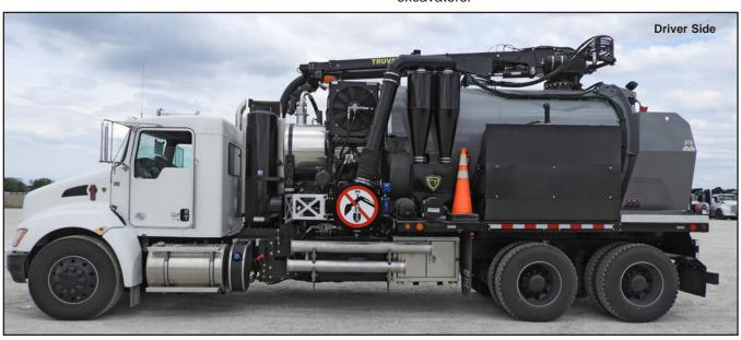
Both mediums have very distinct advantages. Air vacuum excavators use compressed air to loosen the soil and positive displacement blowers to vacuum the spoils into the debris body. Hydro-excavation uses high-pressure water to loosen soils, and the residual slurry spoils are easily extracted into the debris body.
