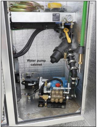
The standard water pump on this unit is capable of producing 10 gallons a minute at 3000 PSI. It is both pressure compensated to ensure the operator maximum performance at a variety of flows or pressures, all through the hand gun.
