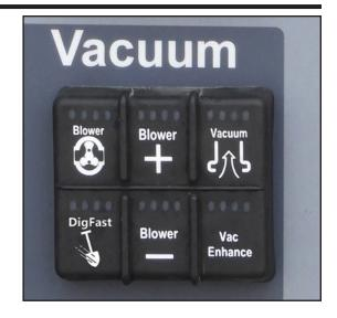
Switch indicator lights. Red will appear for each switch when an E-Stop is activated and blue when enabled.
