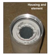
1099061-30 FILTER ELEMENT (includes housing seal). Fill housing with oil before installing.
