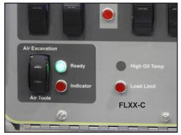
**Air Compressor Option -** Up will activate the air compressor in high pressure mode for excavation, down will activate in low pressure mode for tools.
