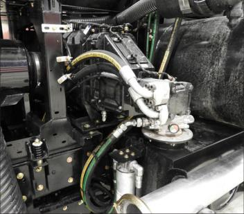
Passenger side blower sight eye can be seen through on the port in the rear of the water cabinet.
