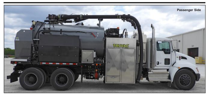
Vacuum Excavation occurs when high-pressure water or pressurized air breaks up and cuts the soil, while a high-flow vacuum system lifts the soil up and out of the excavation area.
