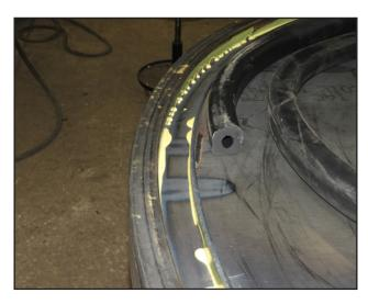
Make sure the end of the seal is cut squarely for a proper seal at the end of the procedure.
