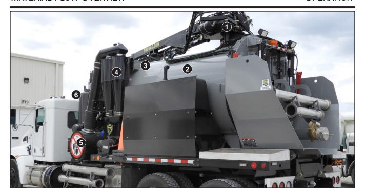
The filtration system is designed to clean the air coming into the system by removing all dirt, dust and foreign matter from the air. The filtration system's primary purpose is to protect the blower by removing all material from the air stream before it reaches the blower.
