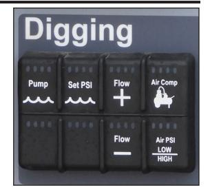
Switch indicator lights. Red will appear for each switch when an E-Stop is activated and blue when enabled.
