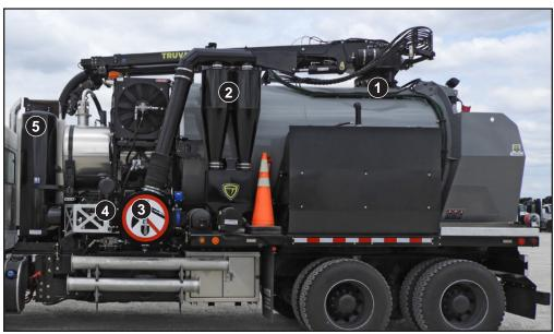
Air leaving the float-ball vacuum shut-off in the debris body enters a cyclone housing. It protects the blower by removing material from the air stream before it reaches the blower.
