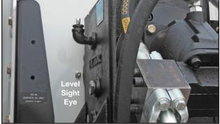
9. After assembly is complete, run the unit for several minutes to circulate oil throughout the box. Shut the unit down. Immediately after the fan has come to a complete stop, check the oil level in the sight gauge. Do this before any oil has had a chance to flow back into the sump. Top off to the midpoint of the sight eye. This oil level should only be checked after the unit has been run.
