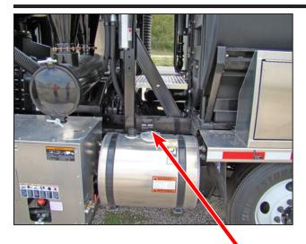
Normal location of Serial No. Plate for HXX units is on the driver side on the front part of the subframe. Options may obscure direct viewing.
