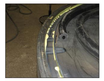
3. Make sure the end of the seal is cut squarely for a proper seal at the end of the procedure. A hacksaw works well.
