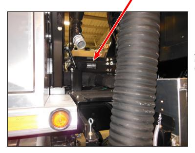
Alternate location of Serial No. Plate for HXX units is on the passenger side under the access steps. Options may obscure direct viewing.
