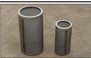
3" Y-strainer on water pump - Disassembled
