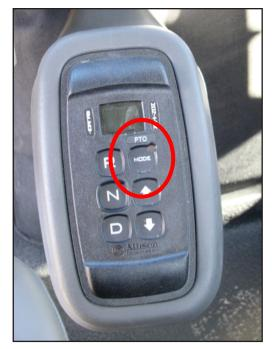
The MODE switch is normally used on automatic transmissions.
