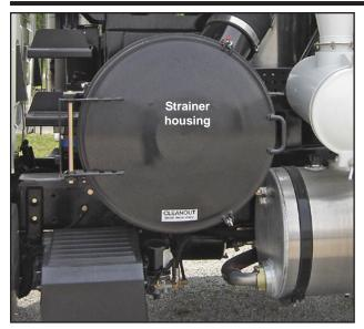
From the cyclone outlet, air enters the strainer housing. The strainer is a perforated screen filter located on the intake side of the blower. Its purpose is to prevent any objects or foreign matter that have entered the system from reaching the blower. The strainer is covered by an automotive style air filter element.
