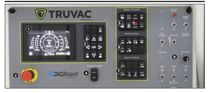
The master control panel containing many of the operator controls is located adjacent to the water tank on the passenger side. The panel is illuminated any time there is power to the master control panel.
