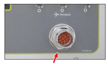
Attach pendant to receptacle on the master control panel
