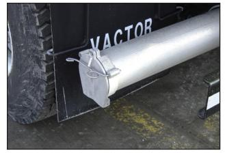
The digging lance and extensions can be stored behind the rear bumper for transport.
