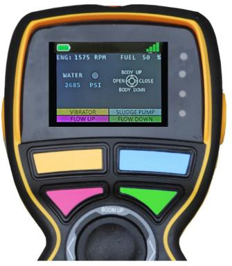
Joystick Functions UP - BODY UP DOWN - BODY DOWN RIGHT - CLOSE REAR DOOR LEFT - OPEN REAR DOOR Button Functions YELLOW - VIBRATOR
