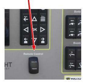
Step 4: Momentarily press the Pair button on the left side of the remote (screen will prompt when needed).
