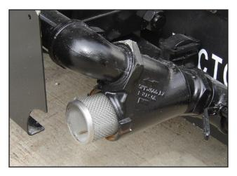
2" Y-strainer at water fill - Disassembled
