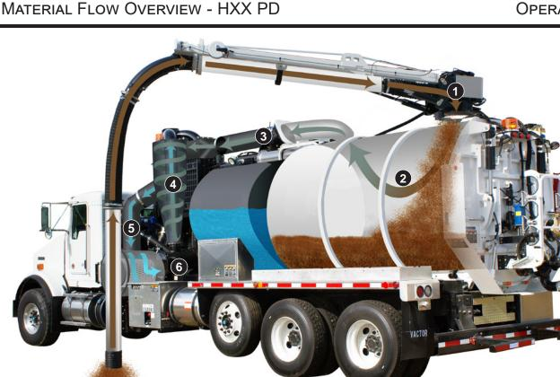
The filtration system is designed to clean the air coming into the system by removing all dirt, dust and foreign matter from the air. The filtration system's primary purpose is to protect the blower by removing all material from the air stream before it reaches the blower.
