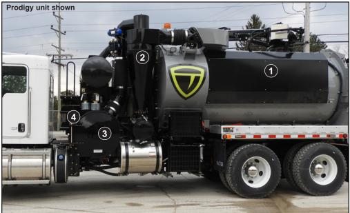
particles toward the cyclone walls where they spiral downward into the collection hopper.
