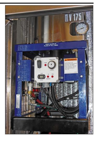
**Burner ON/OFF** - Master switch to operate or shut down water heater.
