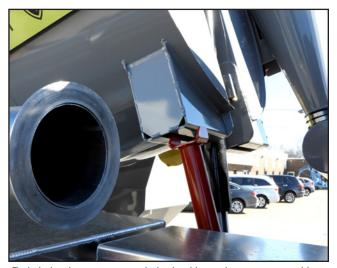
Debris body prop correctly locked in maintenance position.
