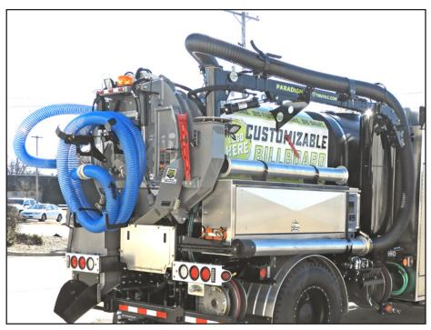
The debris body is equipped with a float ball shutoff. If the body fills with water the float ball blocks the air inlet to stop suction and prevent flooding the blower. This reduces the risk of liquid entering and damaging the blower system.
