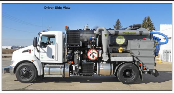
Vacuum Excavation occurs when high-pressure water or pressurized air breaks up and cuts the soil, while a high-flow vacuum system lifts the soil up and out of the excavation area.
