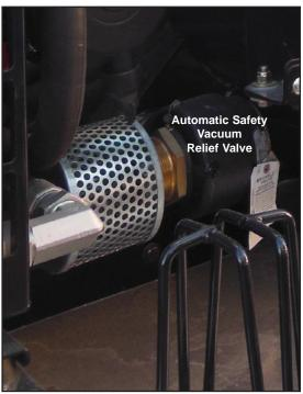
From the debris body, air enters the final filter housing. It's purpose is to prevent any objects or foreign matter which has entered the system from reaching the blower. If it becomes plugged, it will result in a high vacuum and a reduction of air flow. The filter should be replaced if necessary and any foreign matter contained in the housing should be removed.
