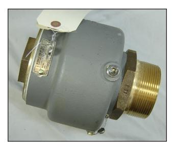
The air operated vacuum relief valve is used to relieve the system if the vacuum hose, debris body or inlet filter become plugged or restricted. These valves are on all blower units. The valves are normally operated from the master control panel, pendant or optional wireless remote. Proper operation should be verified daily by verifying under vacuum. Actual location size and configuration of the valve varies by the model and options. Typical location is in the inlet piping of the blower.
