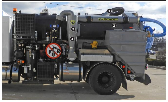
The filtration system is designed to clean the air coming into the system by removing all dirt, dust and foreign matter from the air. The filtration system's primary purpose is to protect the blower by removing all material from the air stream before it reaches the blower.
