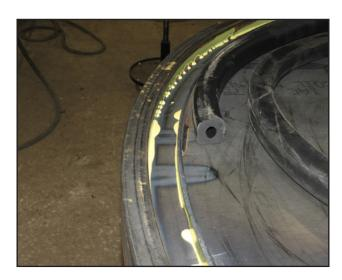
Make sure the end of the seal is cut squarely for a proper seal at the end of the procedure. A hacksaw works well.
