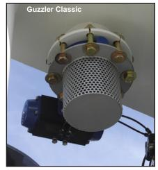
Whether it is manually or automatically operated, a switch energizes an electric over air solenoid valve. This allows pressurized air to fill a chamber on the actuator for the butterfly valve which opens or closes depending on whether the 'on' or the 'off' solenoid is actuated.
