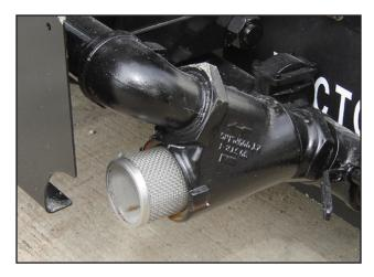
2" Y-strainer at water fill - Disassembled
