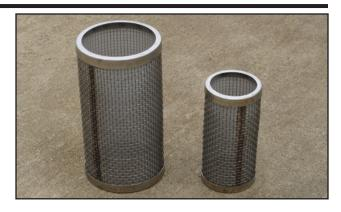
3" Y-strainer on water pump - Disassembled
