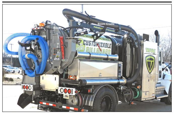
To take the boom out of its stored position, the boom must be raised slightly to clear the boom cradle that it rests upon. Once clear of the cradle, it can be raised, lowered or rotated horizontally.
