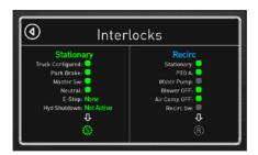
All interlocks need to be green to operate the unit. All PVG valve handle functions are locked out when the wireless remote or pendant is active. Any attempts to use the handle functions while the remote or pendant is in use will stop motion of the function.
