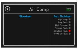
**High pressure shut down** - Unit will go in to shut down after 150 psi is reached.
