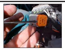
This is a picture of the Terminating resistor. This resistor is also located under the hood. It is 10 to 12 inches from the previous connector. This connector has a resistor installed in the connector and also needs to be checked for corrosion and moisture. Note the terminating resistor must be installed for proper operation. The resistor is sealed under the black cover.
