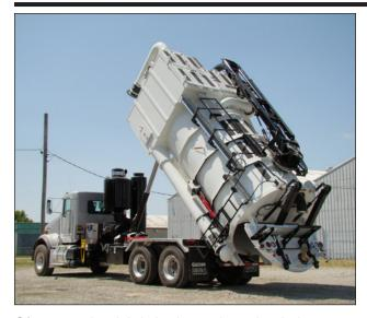
Of course, the debris body can be unloaded conventionally by opening the debris body and raising the tank by means of a hydraulic hoist cylinder.
