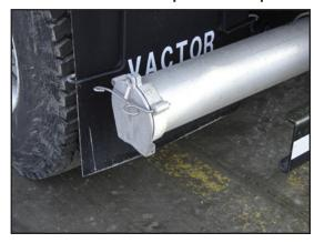
This unit is equipped with a high pressure hand gun. The high pressure hand gun can only be connected to the hose reel located in the water pump cabinet. The high pressure water system uses up to the full water pump pressure of 2500 PSI and can only be used with the special high pressure hand gun or a high pressure wand. The high pressure system also uses a high pressure water unloader valve and ball valve.
