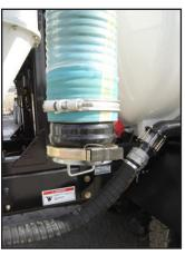
The end of the hose should be capped for travel to prevent debris from sloshing out while moving. Units equipped with a hose keeper do not require this.
