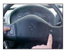
This photo shows the cruise switches, you must depress and hold On and Accelerate simultaneously for a period of 5 seconds. This will bring up the cab diagnostic trouble codes.
