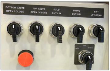
At any time offloading is paused for any reason; including repositioning the cyclone, changing the dump container, the vacuuming should be stopped. If vacuuming is continued uninterrupted, the cyclone might overfill, creating excessive carryover into the baghouse. Additionally, if the manual mode of valve operation is selected, the discharge rate should be at least as fast as the loading rate; not slower.
