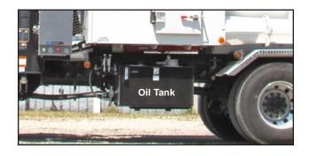
The oil filters supplied by Vactor/Guzzler are equipped with a high efficiency absolute filtering media. Many common filters only give approximately thirty percent filtration of the particles in the hydraulic oil. These filters are referred to as nominal filters. Absolute filtering can give as much as ninety eight percent filtration of the particles in the hydraulic oil. Vactor/Guzzler uses and recommends only the use of absolute filters.
