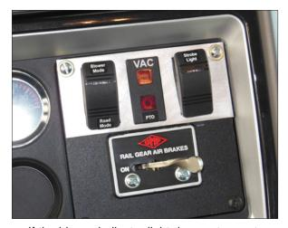
If the blower indicator light does not go out, momentarily press the trans brake switch to allow the chassis driveline to engage.
