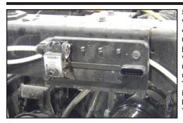
Single valve on 4-valve bank mounting plate. This valve is normally used for the TC/PTO and is located behind the TC.
