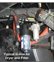
Typical desiccant style air dryer with replaceable filter element.
