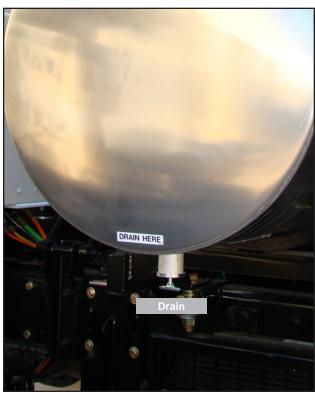
The air purge system uses compressed air to remove water from the water lines, hoses and some components prior to storage in cold weather. The controls are located inside the water pump cabinet.
