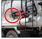
A variety of solenoid valves are used for boom, rear door locks and other options. They are normally located on the driver side towards the rear.
