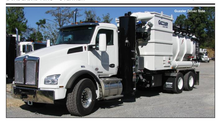
The Liquid Ring industrial vacuum loader combines the best feature of the - high vacuum (28" in-Hg) power, four stage filtration and modular filter components for easy maintenance - with a liquid ring pump. Because of the its unique design, the liquid ring pump is virtually maintenance free and operates at an extremely low noise level.
