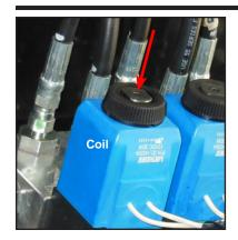
Coils are easily replaced by unscrewing the end cap and removing the wire plug.
