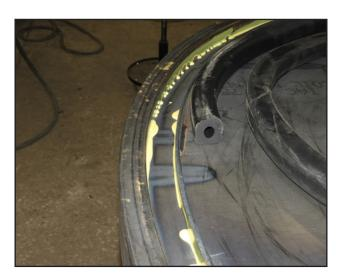
3. Make sure the end of the seal is cut squarely for a proper seal at the end of the procedure. A hacksaw works well.
