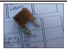
As you can see in this picture there are two very small terminals that the fuse plugs into. Inspect for corrosion and make sure the terminals are still locked in place and not slid back down in the distribution box.
