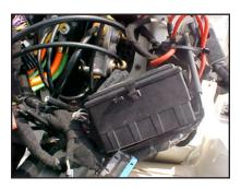
Remove the lid to the power distribution box and look at the diagram on the inside of the lid. Locate the remote power module fuse.
