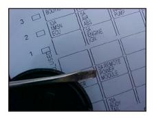
This is the location of the fuse. Remove the fuse and inspect.
