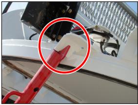
When any work is to be done inside the debris body or on the rear door that requires it to be open, use the rear door support provided.
