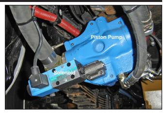
For normal body functions the maximum pressure capability is 2000psi. Maximum pressure for cyclone gate valve operation is 1000psi. The compensator is shifted via an electrical signal.
