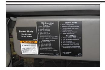
There are several different types of shifters available. Refer to the operating instructions supplied with each truck and the Vactor supplied decal typically on the driver side visor. The common blower shift instructions for manual transmissions is shown for reference. There will also be a designated gear decal on the dash for manual transmissions.
