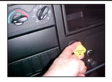
Turn the key to the ON position and wait for the gages to cycle and return to the proper position.
