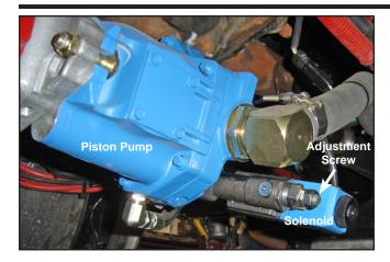
The dual compensator hydraulic system is a variation of the closed center hydraulic system. It is only found on XCR units. These units have a remote cyclone.
