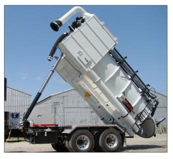
The controls for dumping the debris body are normally located to the right of the master control panel located on the driver side. With the hydraulic PTO engaged run the engine throttle up to about 1200 rpm to operate the control station properly and efficiently.
