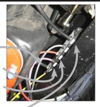
Remote Power Module (Normally located under the driver seat under the cab)
