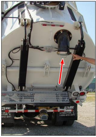
Raise the **empty** debris body to attach vacuum hose to the rear door port.
