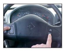
This is how faults are displayed. In this case 2 faults are showing. Continue to watch as the computer will scroll through the faults.
