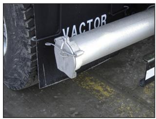
The digging lance and extensions can be stored behind the rear bumper for transport.
