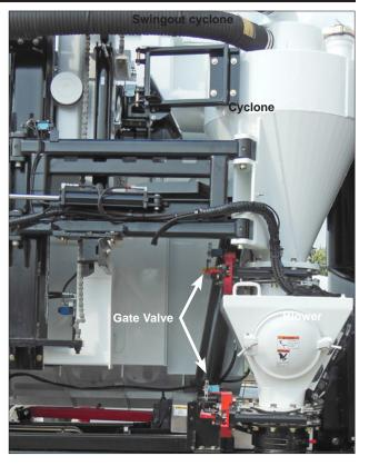
After the debris falls to the bottom chamber, the relatively free air will exit the cyclone through two six inch flexible tubes. Depending on the type of cyclone being used, it will either go to the debris body or will go to the bag house. The opening and closing of the top and bottom valves is either done manually or automatically based upon certain preset time intervals. A three-way switch on the swingout control panel can be set to either the automatic or manual position.
