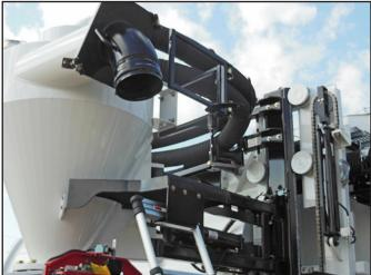
Attach telescoping ladder to the platform hook as shown. Swing the guard rail around and latch in place once on the platform.
