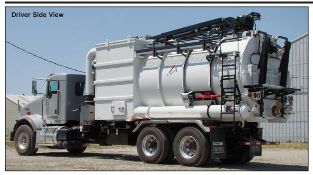
The Guzzler is a powerful, efficient, heavy duty, dust-free, single mode, mobile vacuum loading unit for the pneumatic removal of dry materials, sludges, slurries and liquids from remote and inaccessible locations through suction lines eight inches in diameter and smaller. The vacuum system moves loose material to a debris body for cartage to an appropriate dump or disposal site.
