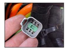
This is what the mating connector should look like. As you can tell there is no sign of moisture or corrosion. You can also see that there is a trace of dielectric grease. This connector should have a small amount of dielectric grease to insure proper connection.
